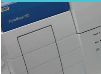
Pyrosequencer - quantitative mutation analysis and DNA methylation profiling
